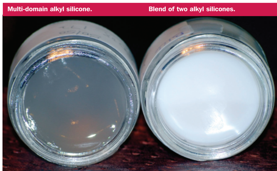
Figure 9: Comparison of multi-domain alkyl silicone and blend of two different alkyl silicone polymers (having the same ratio of alkyl groups).
